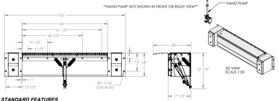
MODEL NUMBER IS PP-2566 OVERALL WIDTH IS 93" **DECK WIDTH IS 66"** OVERALL DEPTH WITH RAMP OUT IS 29" **BUMPER PROJECTION IS 17 1/2"** UNIFORM CAPACITY IS 25,000 LBS. 5" ABOVE / 5" BELOW SERVICE RANGE HYDRAULIC HAND PUMP OPERATION RECOMMENDED FOR DOCKS AT LEAST 48" HIGH. INCLUDES HAND PUMP, WALL-MOUNT BRACKET. CYLINDER, HYDRAULIC LINES AND OIL. TREADPLATE RAMP & DECK CONSTRUCTION
