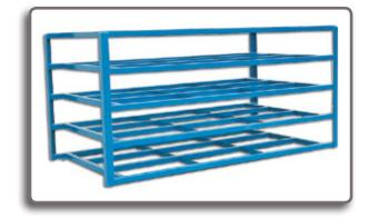
Framing Tech fabricated this 6'x11'x8' sheet storage rack system using 45mm series profiles, 90 series profiles and hard board for the shelves, and blue pvc for the ends. total of 4 units.
