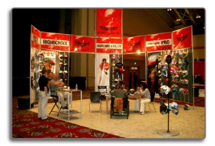
30mm extrusions were used to provide a lightweight yet rigid solution for 12' product displays that had graphics applied as well as product support hooks. The focal point of these sections was an additional 6' high section bolted on top to create an intimidating 18' tall tower effect.
