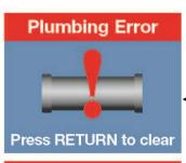
Error caused when SENSOR 1 and SENSOR 2 have been plugged in incorrectly. Swap the SENSOR 1 and SENSOR 2 plug in controller to correct this problem.
