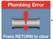
Error caused when SENSOR 1 and SENSOR 2 have been plugged in incorrectly. Swap the SENSOR 1 and SENSOR 2 plug in controller to correct this problem.
