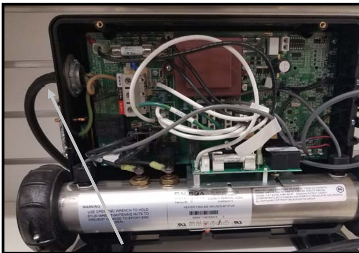
Add strain relief here
