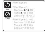
At the start of each filter cycle, the water will run briefly to purge the plumbing to maintain good water quality.
